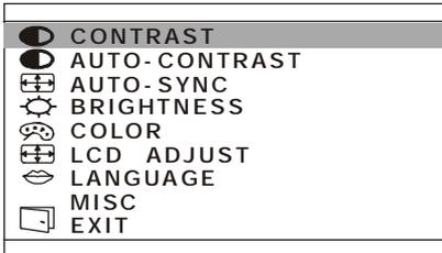
**CONTRAST** adjusts the foreground white level of the screen image. Under Main Menu, select CONTRAST using the **[+]** or **[-]** button, then press **Menu** button to activate the function. Press the **[+]** button to increase contrast, **[-]** button to decrease contrast. Press **Menu** to return to Main Menu.
